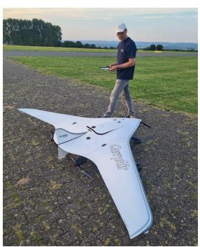
With the rising twilight, Thomas starting to prepare his new big commercial drone. Thomas, one of the "Silence-Brothers", currently designed a very special drone for commercial purpose. The concept is a bit different to the main stream. The drone can act like a standard drone and like a standard plane. Thanks to this, the payload and operating time is much better than many other drones on the market.
