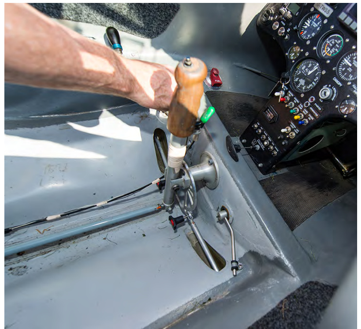
Top It's a pretty spacious single seater, note FLARM display at top of panel Above Easy access for rigging with the seat removed. Wing pins lock into place with an over centre twist motion. Note also trim lever on the stick Right Here lies fire! Buttons to set the wingtip pyros off when fitted for a display
