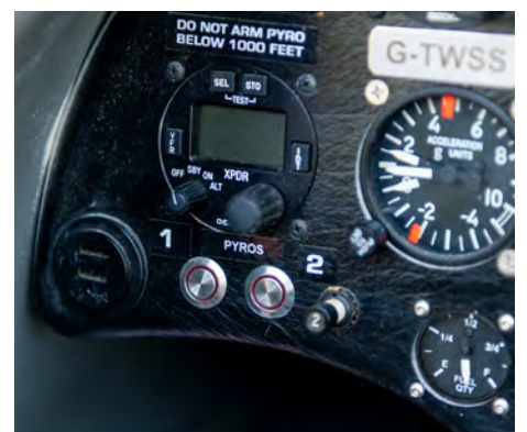
Top It's a pretty spacious single seater, note FLARM display at top of panel Above Easy access for rigging with the seat removed. Wing pins lock into place with an over centre twist motion. Note also trim lever on the stick Right Here lies fire! Buttons to set the wingtip pyros off when fitted for a display
