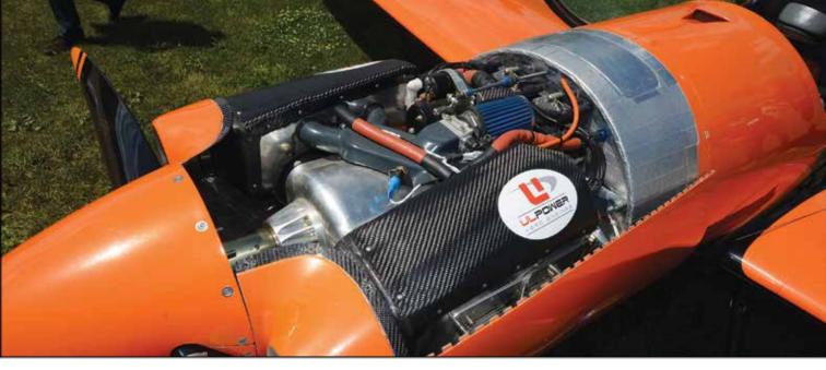
Looking for reliability in a compact form, Andy opted for ULPower's UL260iSA 4-cylinder. The aerobatic engine boasts fuel injection and raised compression to make 107 hp from just 2.6-liters (159 cubic inches). The carbon fiber plenum cooling is Andy's own work. As for expense, the ULPower mill cost about \$20,000 in round numbers, or "Certainly not as expensive as the iS version of the Rotax."
