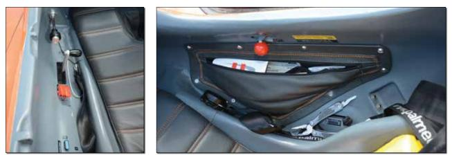
(Left) The vernier control on the cockpit's left side is for elevator trim. Twin red power bus toggles are aft of the throttle, and the teal handle is for the parking brake. (Right) Storage is what's going on to the right in the cockpit. The pliers handle partially covers the cowl flap control, the red knob is the canopy latch, and the headset jacks are self-evident at the lower right.
