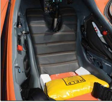
Even with the custom 6-gallon "headrest" tank, there's still storage room in the turtle deck. Only the top of the tank is visible here; it forms the headrest storage area floor. Fuel in this tank gravity flows to the left main tank, leading to a notably aft CG until this aft-most tank is emptied.
