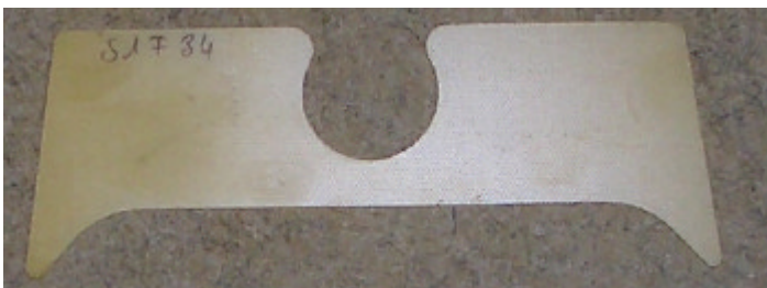
Fig. 2.3.3.2 Support rib needs to be installed 10mm before the end of the rear tube with a 5mm radius of cotton flox resin.
